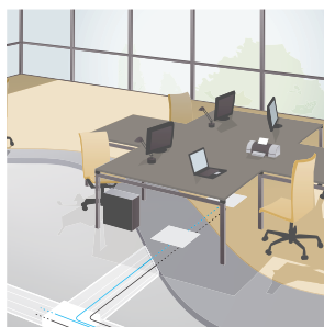
Screed floor system
