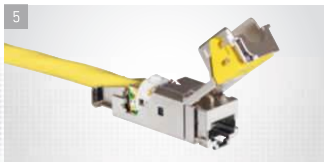
Install the wire housing without pushing
