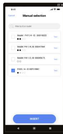
Association of a thermostat to the corresponding actuator
