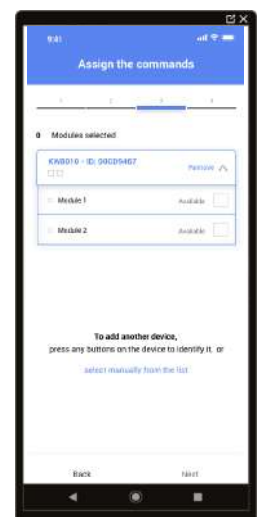
Association of a thermostat to the corresponding actuator
