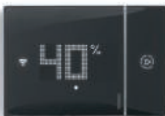
Display the set room temperature and humidity
